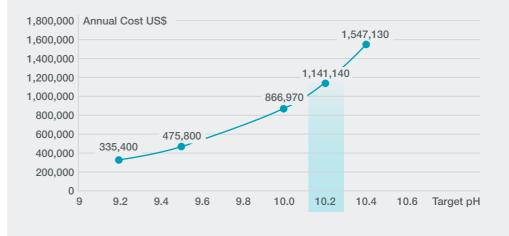
pass is through a second pass where the pH is raised to above 10 using sodium hydroxide (NaOH), increasing complexity and cost, and environmental footprint.
